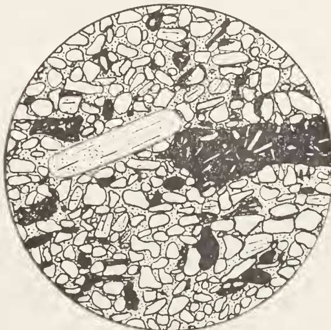
Fig. 4.—Sandstone (specimen 38716) showing feldspar grains (stippled, with cleavage), volcanic fragments (dark) and quartz grains (clear) in an abundant matrix. Diameter of field, 2 mm.
